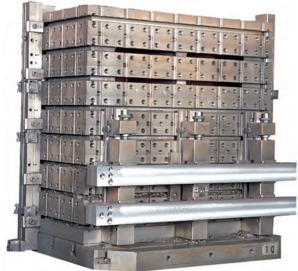
Horizontal application; three Flex-Clamps with multiple intermediate blocks.
