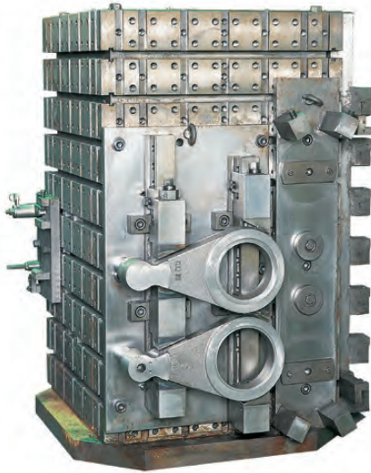
Horizontal application; Flex-Clamps: #1 with an intermediate block and formed jaws. #2 with formed jaws on both the intermediate, moveable and fixed jaws.
